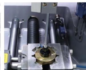
Automatic Sample Height Measurement System
