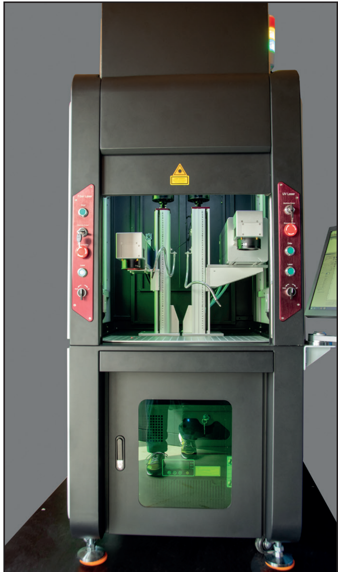
On the left you can see the fibre laser, on the right the UV laser
