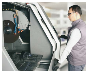
Two Hand Control For Safety Operation
